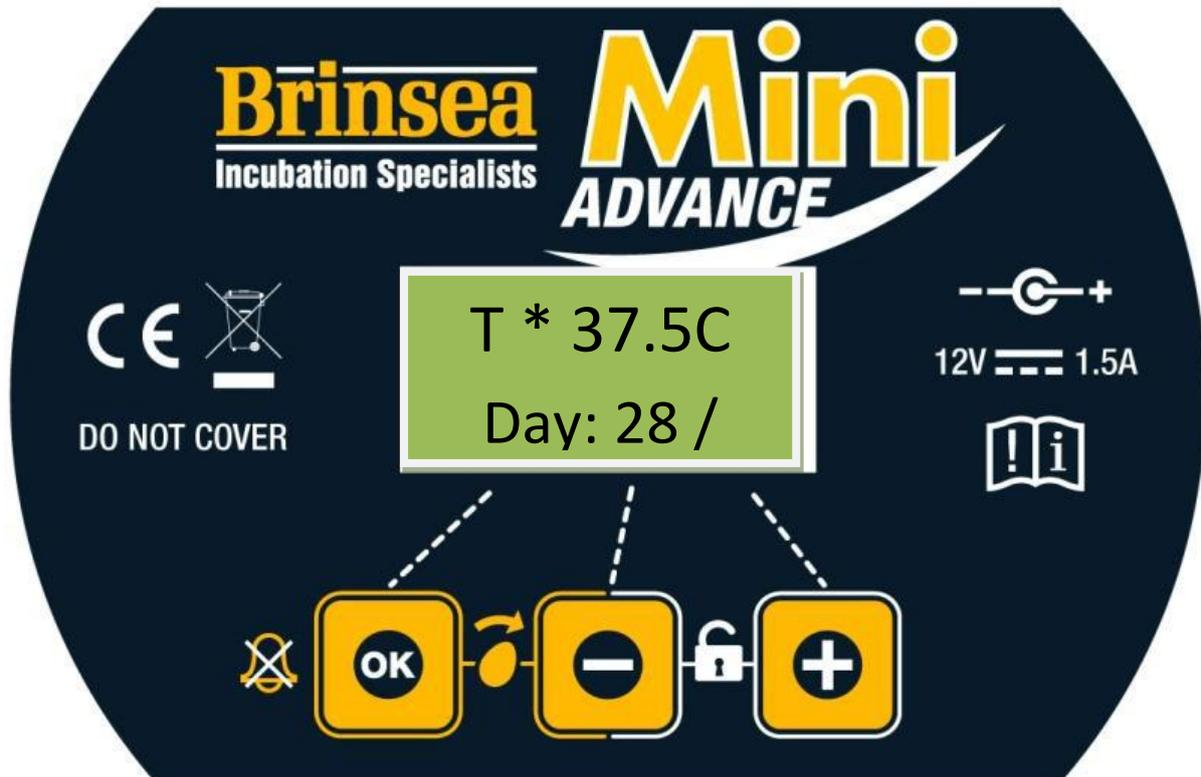
Normal operation – Temperature, number of days remaining until the hatch is due and turn system status are continuously displayed.
